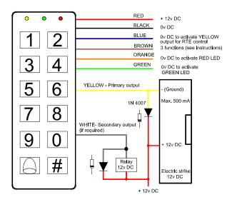
Electric strike, supplementary relay and additional diode shown in the above circuit diagram are for illustrative purposes only and are not included with the CT 1000. Please order separately.
